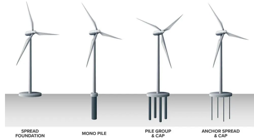
Different onshore wind turbine foundation types
